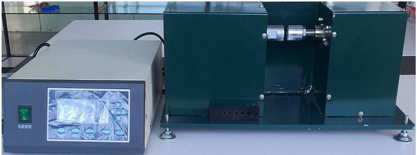
Connect the power 220V, connect the signal line plug between the power supply and the main engine.
