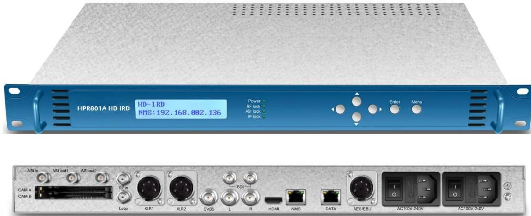
HPR801A HD IRD support AVS+/H.265/H.264/MPEG2 video decoding and DRA/AC3/EAC3/AAC/MPEG audio decoding. It support DVB-S/S2,DVB-T/T2,DVB-C tuner/ASI/IP input and 1080P/1080I/ 720P/576I/480I output resolution.The two CAMs/CIs accompanied and BISS modules can descramble the programs input from encrypted Tuner, ASI and IP.
