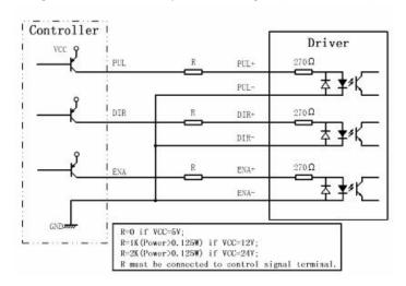
Figure 4: Connection to PNP signal (common-cathode)
