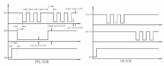
Figure 11: Sequence chart of control signals
