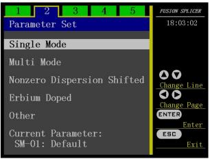
Press " $\blacktriangle$ " " $\lor$ " to move the cursor, and press "ENTER" to enter the "Fusion Splicing Mode" program that you want to get into.
