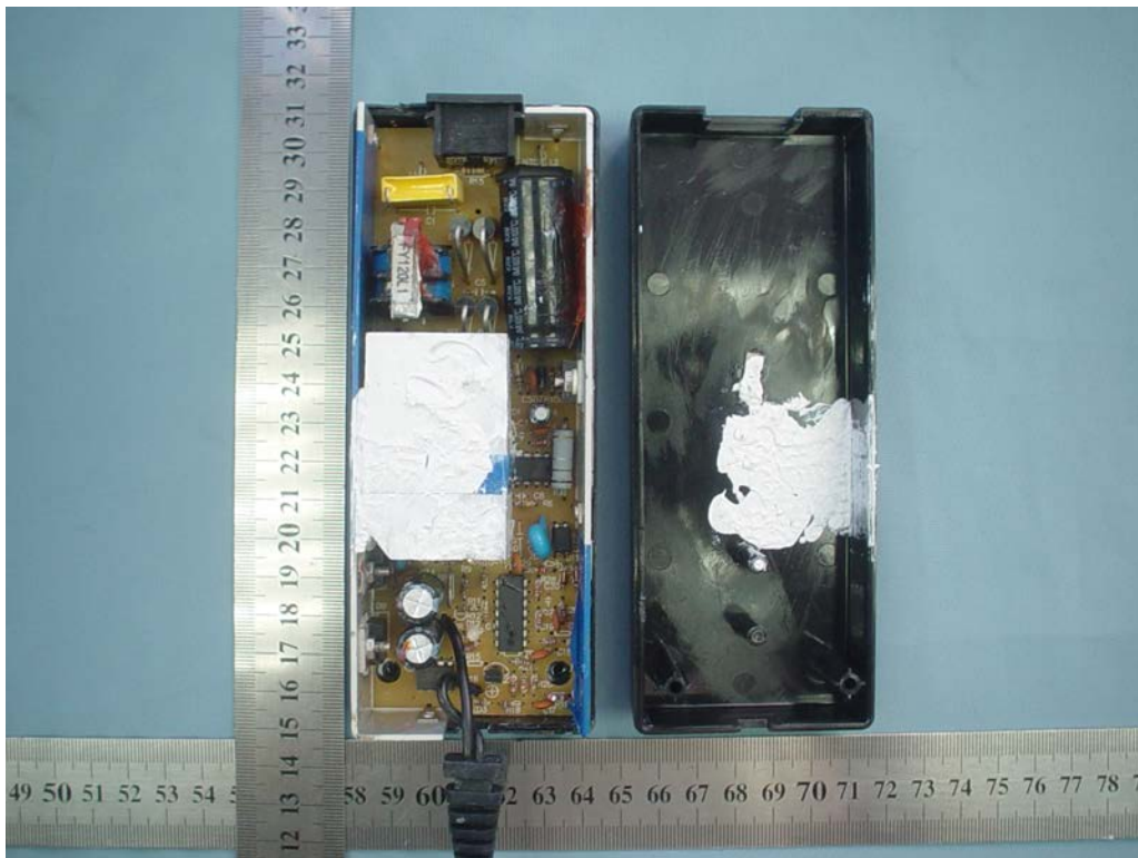
Figure 4. top view internal circuits
