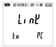
Attention! The transmission speed should be 9600 baud (please refer to user manual of application software). Please connect this instrument to PC according to Figure 7.
