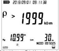
Soil resistance coefficient beyond measuring range during soil resistance coefficient measurement
