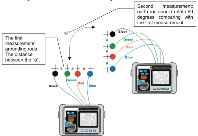
Soil resistance coefficient should be calculated according to this formula:
