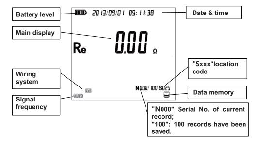
START Press "START" to start measuring and reading measured value. After measurement, the screen will show the following:
