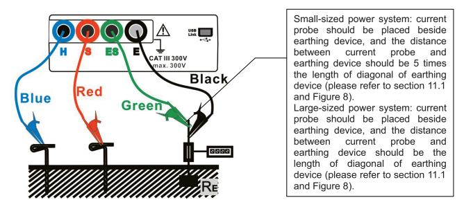
Figure 4. Earthing 3 Wires for Resistance Measurement
