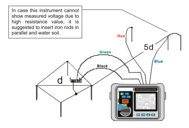
Figure 8. Measure Earth Resistance with Voltmeter-Ammeter (Small-Sized Earth Screen)
