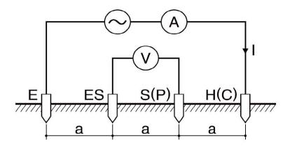
Figure 5. Method of Calculating Soil Resistance Coefficient (ρ)
