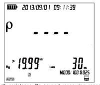
Earth resistance Rg beyond measuring range during soil resistance coefficient measurement
