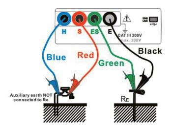
Figure 3. Earthing 2 Wires for Resistance Measurement
