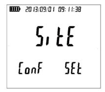
1. ENTER Press "ENTER to start setting measuring position, and the screen will show the following:
