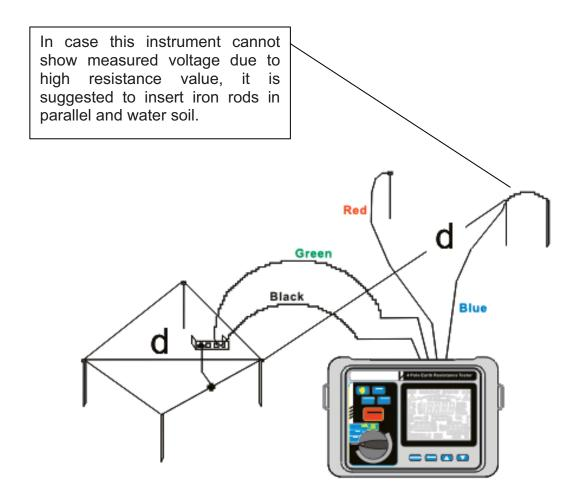
Figure 9. Measure Earth Resistance with Voltmeter-Ammeter (Large-Sized Earth Screen)
