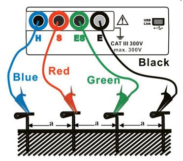
Figure 6. Earthing 4 Wires for Measuring Soil Resistance Coefficient
