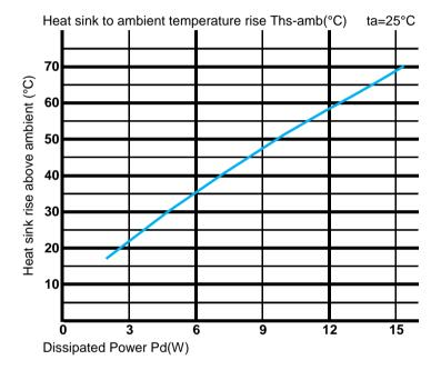
\*The aluminum substrate side of the package outer shell is thermally connected to the heat sink via TIM (Thermal interface material). MingFa recommends the use of a high thermal conductive interface between the LED module and the LED cooler. Either thermal grease, A thermal pad or a phase change thermal pad thickness 0.1-0.15mm is recommended.
