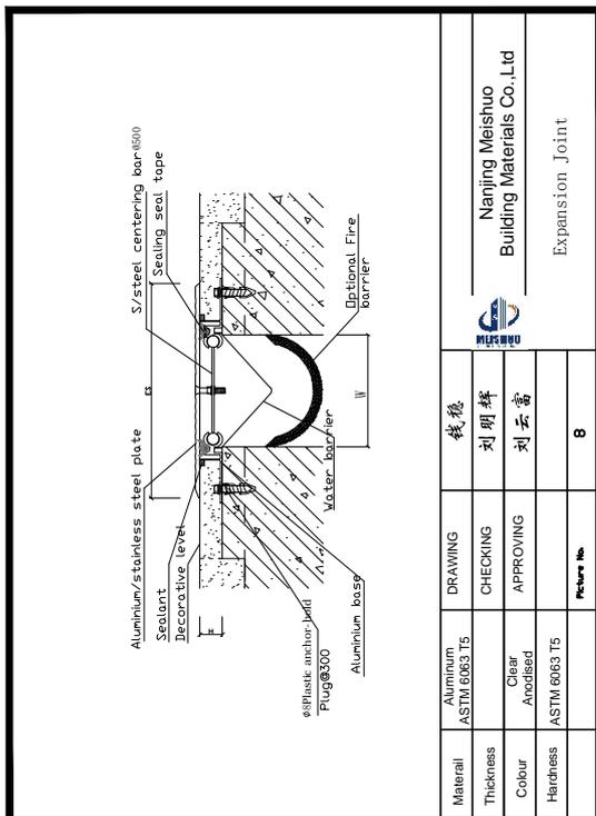
7. Nail the scree to make sure the base on a straight line. Or the aluminum plate can be mismatched when the centering bar bolt is screwed down,
