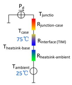
\*Thermal resistance is a heat property and a measurement of a temperature difference by which an object or material resists a heat flow. Geometric shapes are different, the thermal resistance is different. Formula:  $\theta = (T_{hs} - T_a) / P_d$
