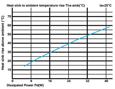
\*The aluminum substrate side of the package outer shell is thermally connected to the heat sink via TIM (Thermal interface material).
